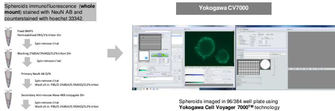
**Fig 1. Methods for imaging and analysis of spheroids using SpheroMatrices spheroid tissue microarray (TMA) technology versus whole mount confocal imaging technology (Yokogawa Cell Voyager 7000 ).**
